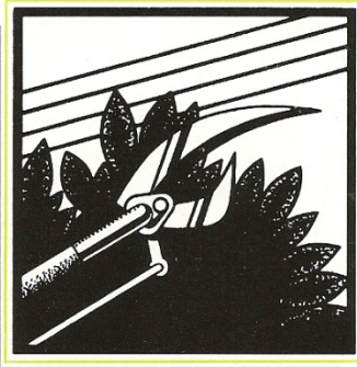
Never trim trees near overhead lines.
